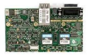
The Ethernet System Interface has both an RJ45 Ethernet connection and an enhanced 15-way D-range. Link selectable radio interface signals include balanced and unbalanced audio, E&M, four bi-directional I/O lines, Rx gate, Tx key, coax relay and RSSI.
